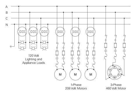
In this illustration, however, loads are unevenly divided. A large number of lighting and small appliance loads are connected to phase C . This can cause the voltage on phase C to be lower. Because a small unbalance in voltage can cause a high current unbalance, overheating can occur in the C phase winding of the 3-phase motor. In addition, the single-phase motors connected to phase C are operating on a reduced voltage. These loads will also experience heat related problems.
