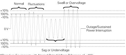
\*Based on Equipment with Normal Rated Voltage Tolerance of ±10%
